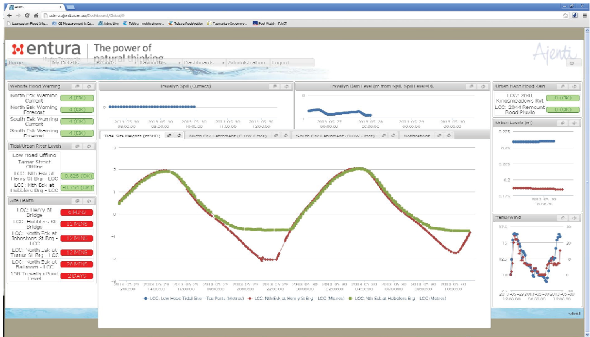
C: Screenshot of the ADMS showing a typical dashboard for hydrometric sites plots, alarms and notifications
